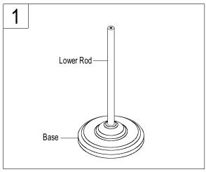
1. Place base on a flat level surface and thread lower rod onto base in a clockwise direction.
