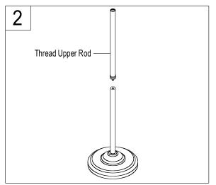
2. Thread upper rod onto lower rod, the end that has the decorative ring should be facing down.
