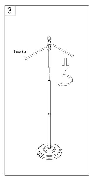
3. Install towel bar assembly onto rod by threading assembly in a clockwise direction.
